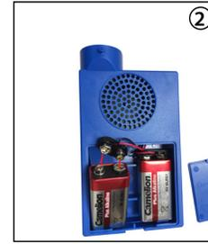
Ensure placement is matching battery (+ positive & - negative)
