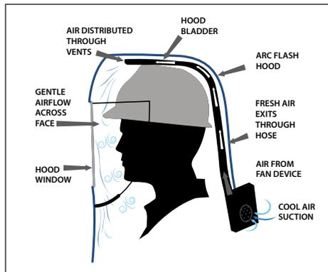
**Fan Fitting & Air Flash Hood Ventilation System Instructions**
