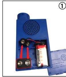
Insert batteries facing upwards
